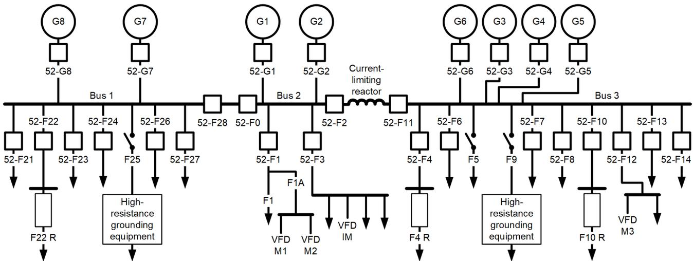
Fig. 1. Red Dog Mine load-shedding scheme
